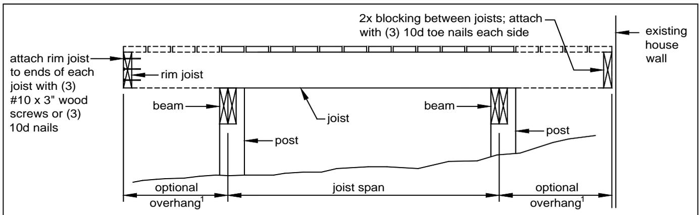
**FIGURE 4: JOIST SPAN - FREE-STANDING DECK<sup>2</sup>**
