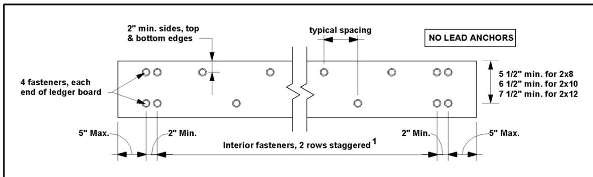
**FIGURE 20: LEDGER BOARD FASTENER SPACING AND CLEARANCES**
