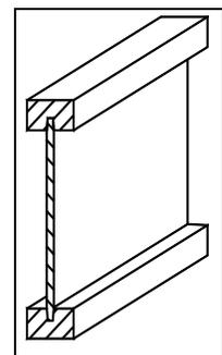
**FIGURE 13: WOOD I-JOIST PROFILE**
