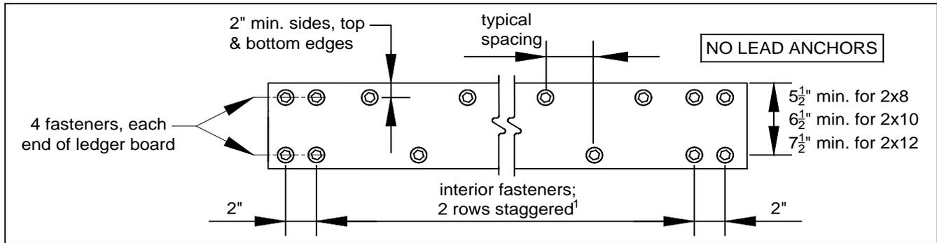
**FIGURE 20: LEDGER BOARD FASTENER SPACING AND CLEARANCES**
