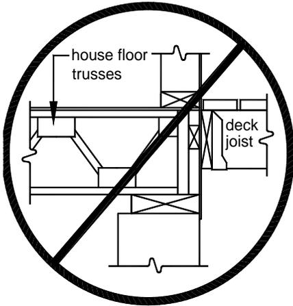
**FIGURE 17: FLOOR TRUSSES**
